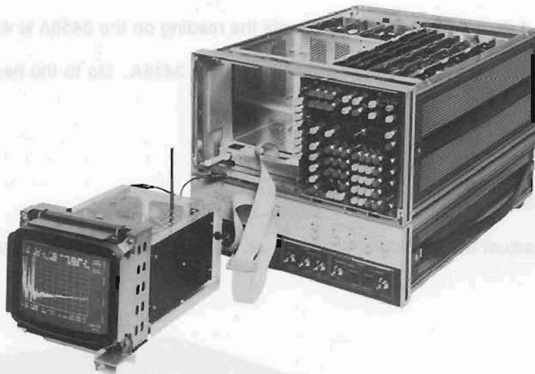
Figure 5-43. Local Voltage Regulator Adjustment Setup
