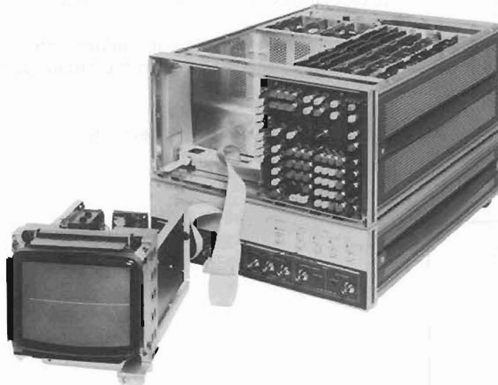
Figure 5-46. CRT Cutoff Adjustment Setup
