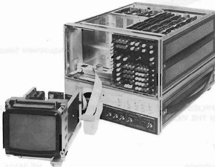
Figure 5-44. Horizontal Position Coarse Adjustment Setup
