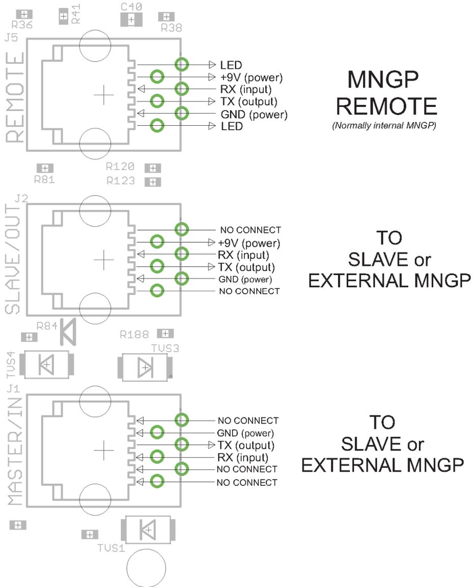
Figure 1. Classic RS-232 MODBUS RJ-11 PHONE JACK PINOUTS (Top View)
